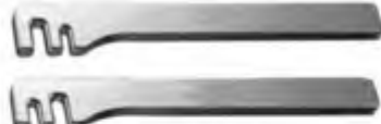
Bending Iron for plates 2.7 and 3.5 Length 150mm, slid widths 2.5 and 4.5mm, required pairs Item Slid placement 054-210 4.5/2.5mm 054-211 2.5/4.5mm
